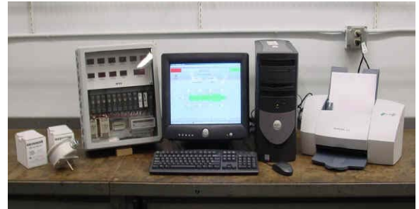
CMCP5000 System With Desktop PC Running Wonderware InTouch® HMI Software
